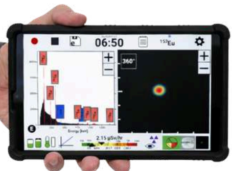
Remote control acquisitions using Real-Time Software on the tablet.
