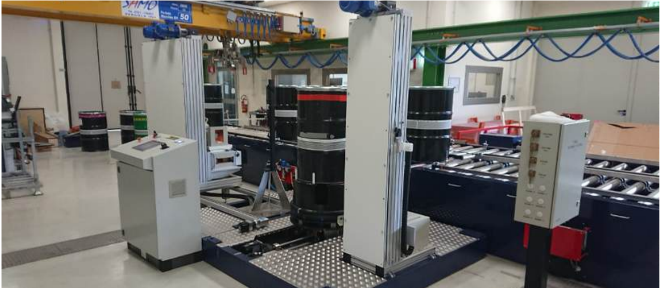
Segmented Gamma Scanning station by Syscade, JRC Ispra, Italy
