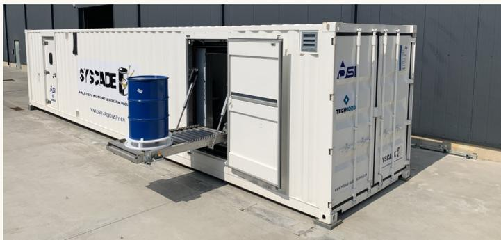
DSi, Scannix and Technord joined their expertise to develop a mobile unit for radioactive waste drums analysis, both physically (drum contents) and radiologically (qualitative and quantitative analysis of the isotopes present in the drums).
